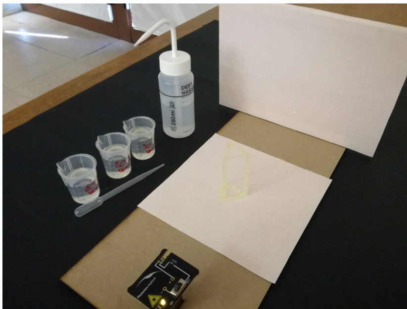
Figure 3.5: Outline vision of the set-up mounted with the materials needed for the determination of sugar content.
