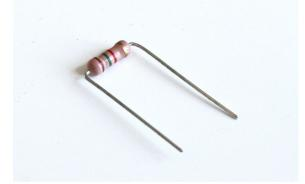
Then, place it in the holes that have the value of the component printed. For these resistors: check the colour codes carefully to make sure it is the right one.
