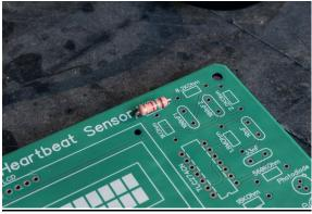
To make your life a lot easier, you can bend the leads over. This makes the component stay in place while soldering.
