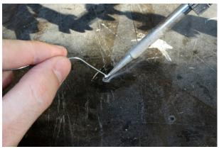
Hold the soldering iron to the lead and the PCB so they heat up. Then, apply solder to the components (not the iron).
