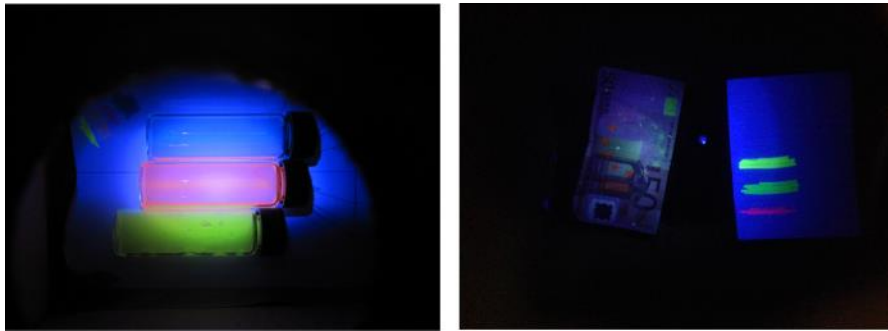
Fig. 9 Fluorescent samples showing some fluorescent paints dissolved in water, a bank note and fluorescent highlighter marker on white paper.
