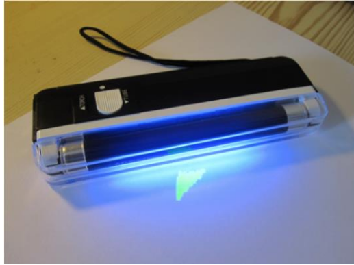
Fig. 7 Image of the hand held note checker or 'black light' which is the UV light source used in this workshop. This is used for viewing fluorescent samples such as yellow highlighter ink as shown on the white page.
