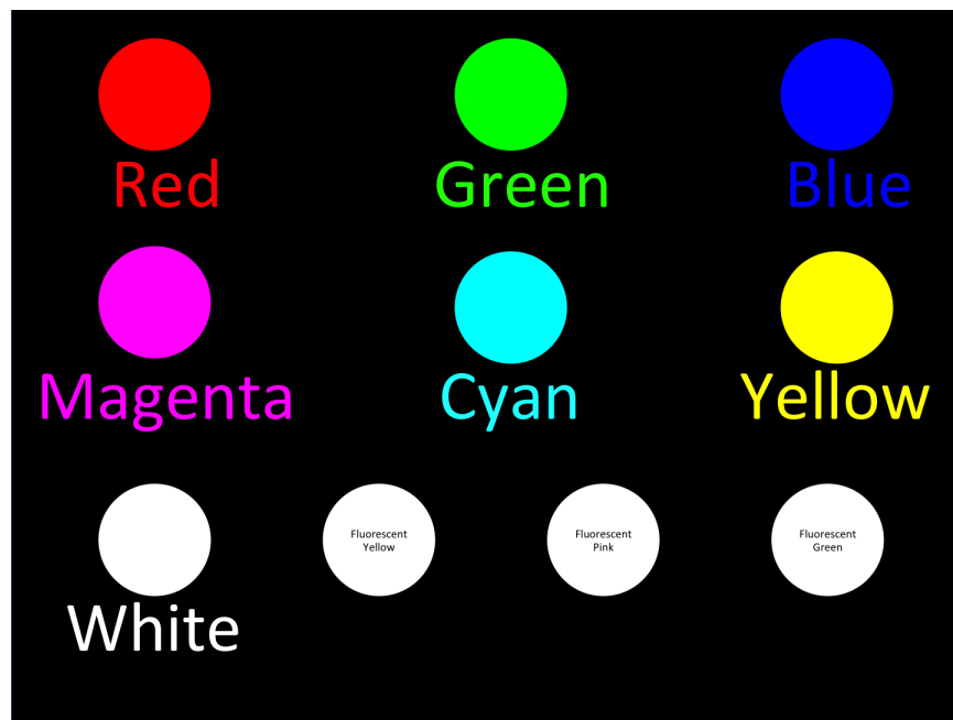
Fig. 6 The colour target which will be printed. The three circles at the bottom can be coloured in after printing using fluorescent markers using Yellow, Pink and Green highlighters pens. These are the fluorescent samples.
