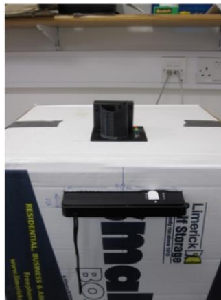
Fig. 4 Image of the box which acts as a 'dark room' to block ambient light.
