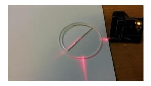
Since  $\alpha_L = \arcsin(1/n)$ , we can use  $\alpha_L$  to estimate  $n = 1/\sin(\alpha_L)$ . Obviously the three different estimations must coincide (unless measurement errors).
