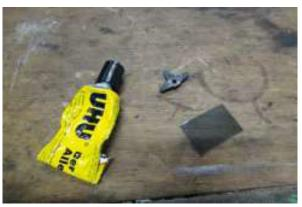
Cut out a small piece from the polarizer foil. In our case a rectangle of 4cm x 2.5cm was sufficient. Additionally, we rounded up two corners to ensure that the polarizer can be turned freely above the ground of the casing. Glue the attachment to the polarizer, either by using double-sided tape or normal adhesive.
