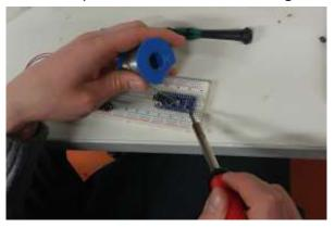
Be careful not to create any solder bridges as those can compromise the functionality of your polarimeter or even damage the Arduino. If unsure, use a multimeter to measure the resistance between two pins. It should be a high value (at least 1  $M\Omega$ ).
