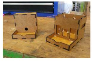
Once you know which parts belong together, glue the different parts together. Please note: The topmost lid of the bigger of the two casings must not be glued to the rest as we will have to embed the electronics later.
