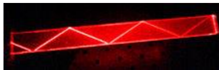
Fig. 7 : Light guidance using laser in a plexiglas sheet where the lateral side have been polished.
