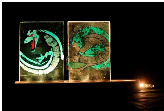
Fig. 8 : Drawing directly on the plexiglas surface (left) versus drawing on a transparent slide placed on the plexiglas surface (right). We use water in the right case to get an optical contact between the plexiglas and the slide.
