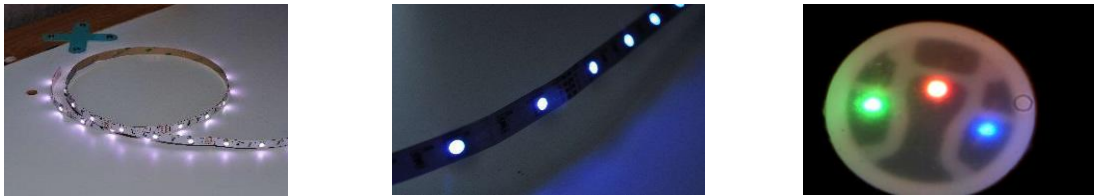
Fig. 15 : Typical LED ribbons
