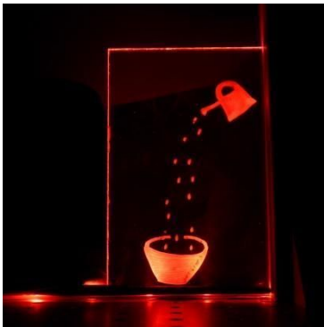
Example 3 : Application of the principles of fluorescence : The flower stalk is made of fluorescent pink that appears both on green and blue light, while the flower petal appears only with the blue light.
