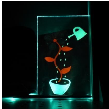
Example 3 : Application of the principles of fluorescence : The flower stalk is made of fluorescent pink that appears both on green and blue light, while the flower petal appears only with the blue light.
