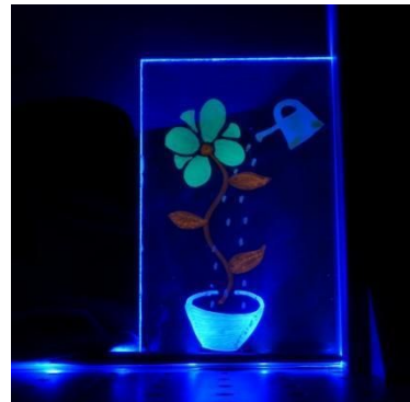
Example 3 : Application of the principles of fluorescence : The flower stalk is made of fluorescent pink that appears both on green and blue light, while the flower petal appears only with the blue light.
