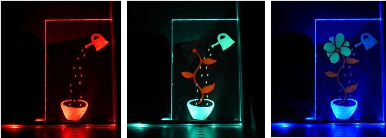
Animated drawing using RGB lighting of an image combining classical and fluorescent inks.
