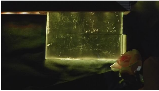
1/ Two slices of adhesive tape on the Plexiglas light guide surface
