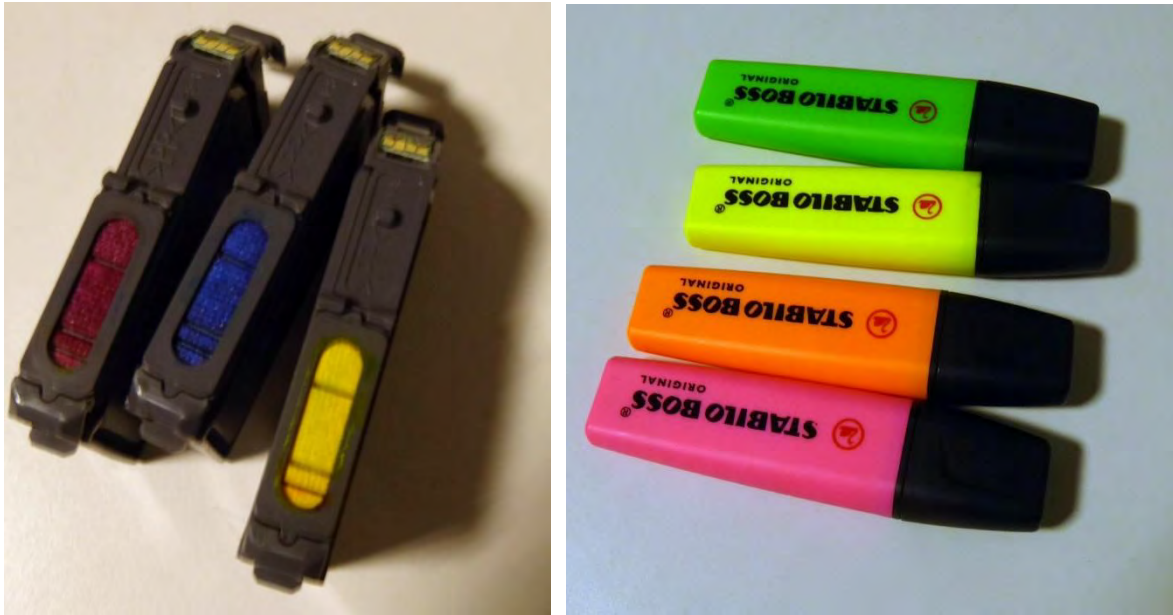
Figure: (left) cyan, magenta and yellow well-worn inkjet cartridges used to produce the colored samples, by collecting some ink with a paintbrush; (right) Fluorescent highliners
